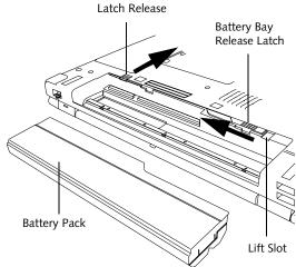
Figure 4-1. Removing a Battery
